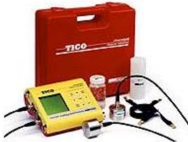
Fig 5: Apparatus for UPV measurement
